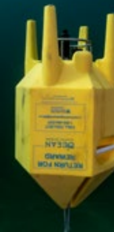
An OTN receiver unit encased in a custom float collar. Nicolas Winkler Photography
