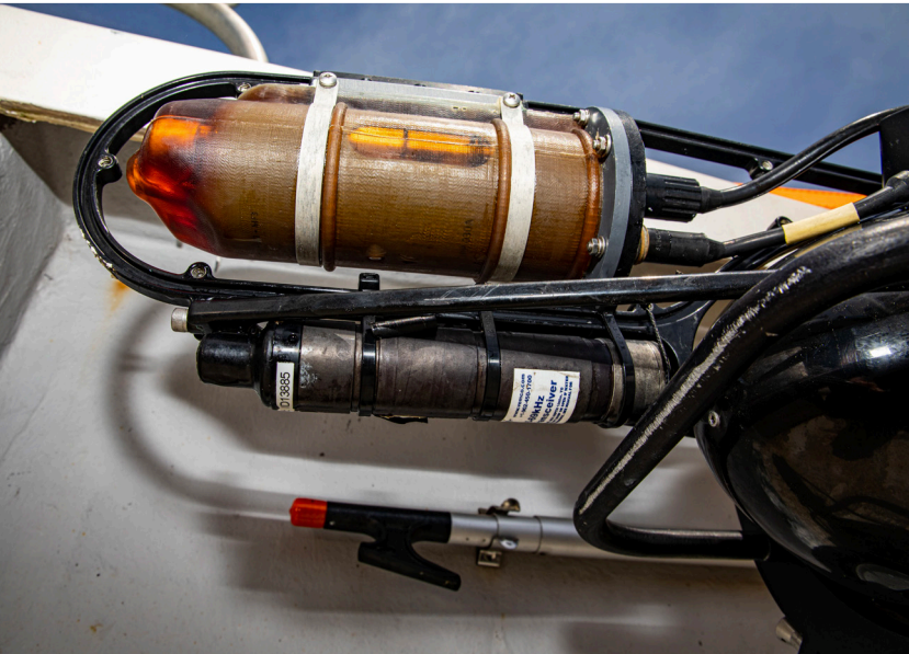
A Slocum glider equipped with a hydrophone that listens for whale calls and a transceiver—a tracking unit that acts as both a transmitter and a receiver.
