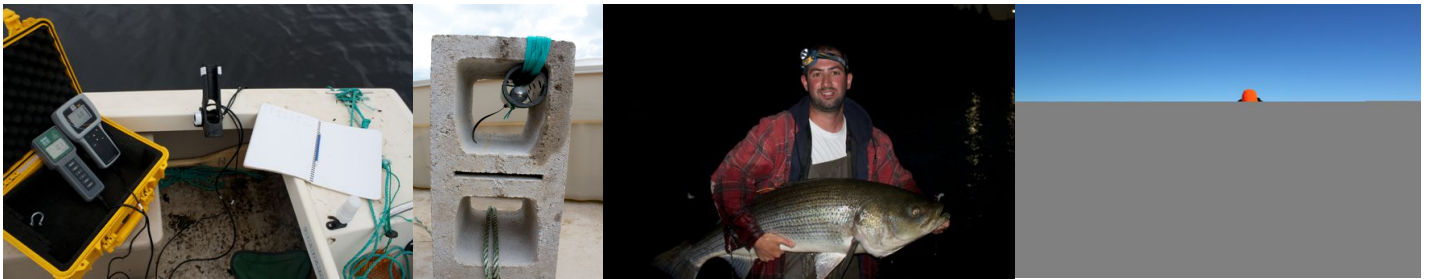
Figure 5. From left to right: YSI 63 and 550a meters used to measure temperature, salinity, and dissolved oxygen; Hobo water level logger in mooring; largest Striped Bass acoustically tagged in Mira system; Using VEMCO VR100 to locate the overwintering site in February 2014
