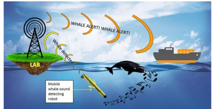
**Whale-alert system:** Autonomous robot "glider" detects whale locations and transmits the data to the lab via satellite. Data are used to alert ships to the presence of whales via an AIS Aids To Navigation transceiver via our cell-tower network.
