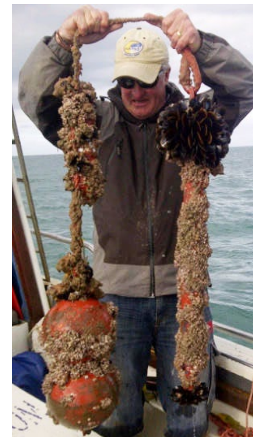
VR2W mooring with extensive biofouling recovered in Algoa Bay, South Africa
