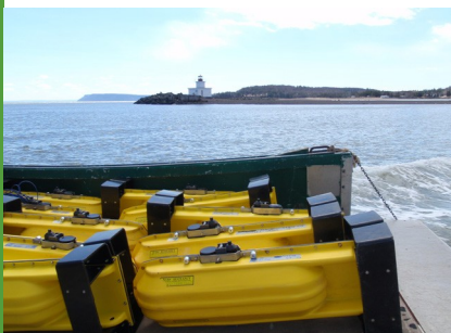
Unique mooring assembly designed to withstand extreme tidal currents in Passage (see Tech Talk p. 8)
