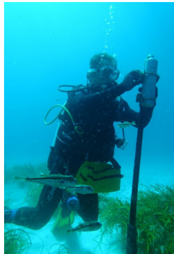
Nick Jarvis uses SCUBA to service receiver on shallow water mooring
